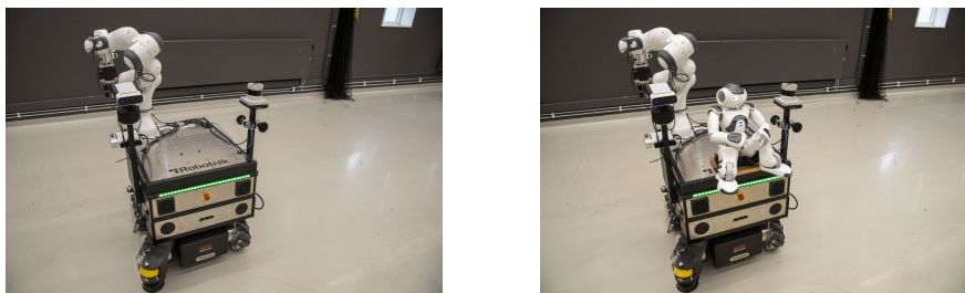
Figure 8: Left: The DARKO robot in the factory stage appearance is called "Robot 1 in its current appearance". Right: The DARKO robot with the humanoid-looking robot NAO (from SoftBank Robotics) on top is called "Robot 2 with humanoid robot."
