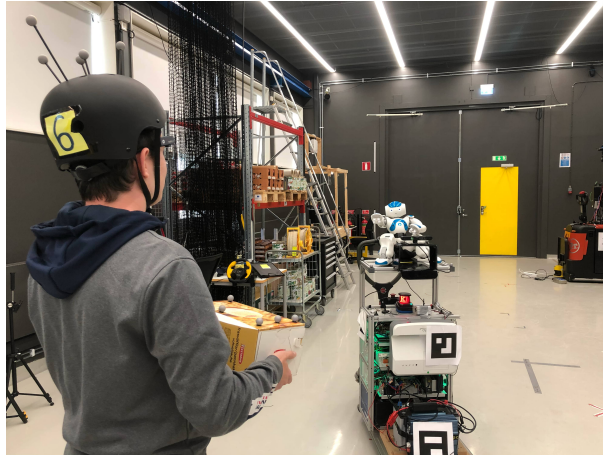
Figure 10: In Experiment A, participants interact with a robotic forklift. The ARMoD instructs the participants to place an object on the forks of the mobile robot.
